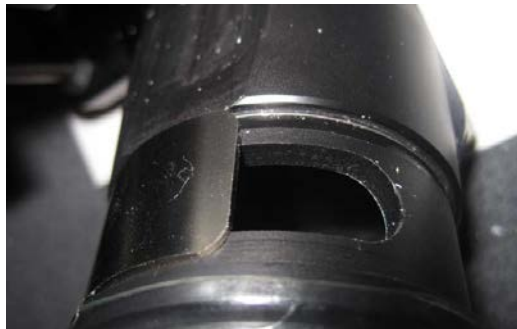
FIG 2-82 RING TO SET THE VACUUM STRENGTH
