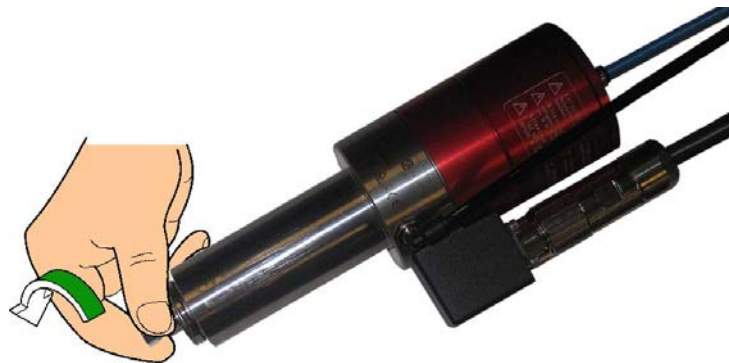
FIG 5-10 REMOVING COLLET FROM THE MILLER
