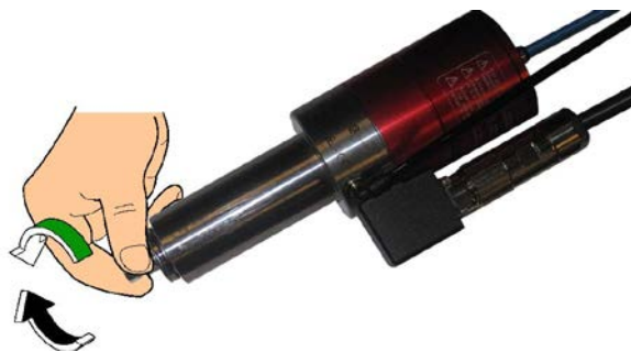
FIG 5-13 RE-INSTALL THE COLLET FROM THE MILLER
