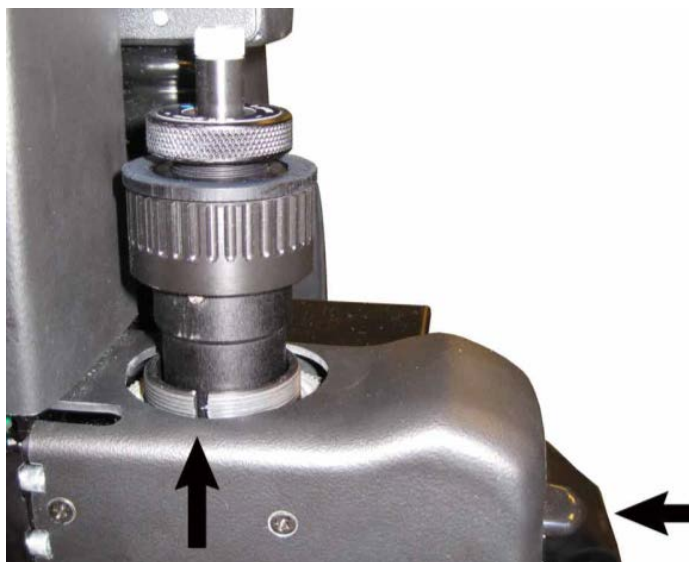
FIG 2-14 INSERT THE KISS CUTTING TOOL
