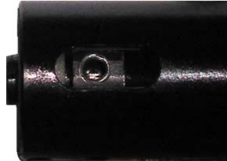
FIG 1-30 KNIFE HOLDER SHAFT – SETSCREW REMOVED FROM EOT
