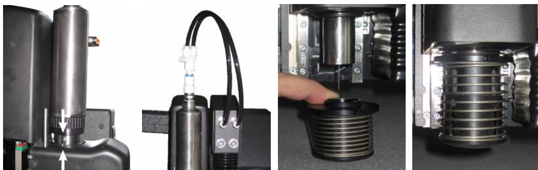
FIG 2-18 MOUNTING THE POT
