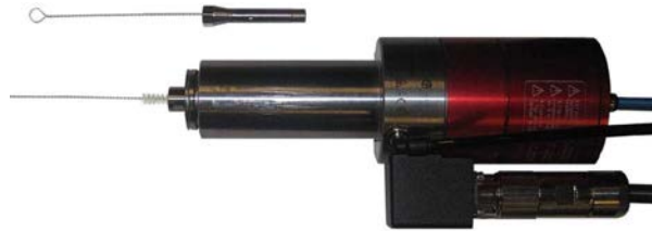
FIG 5-12 CLEANING THE COLLET
