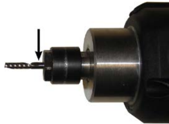
FIG 2-26 ROUTER BIT POSITION ON THE COLLET
