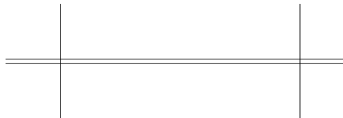
FIG 2-65 TEST PATTERN KNIFE DEPTH TEST V-CUT
